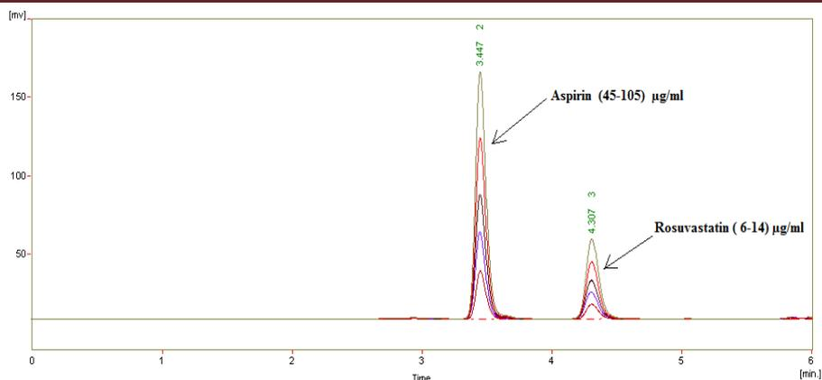
Figure 2: Chromatogram of Aspirin and Rosuvastatin Calcium Mixture
