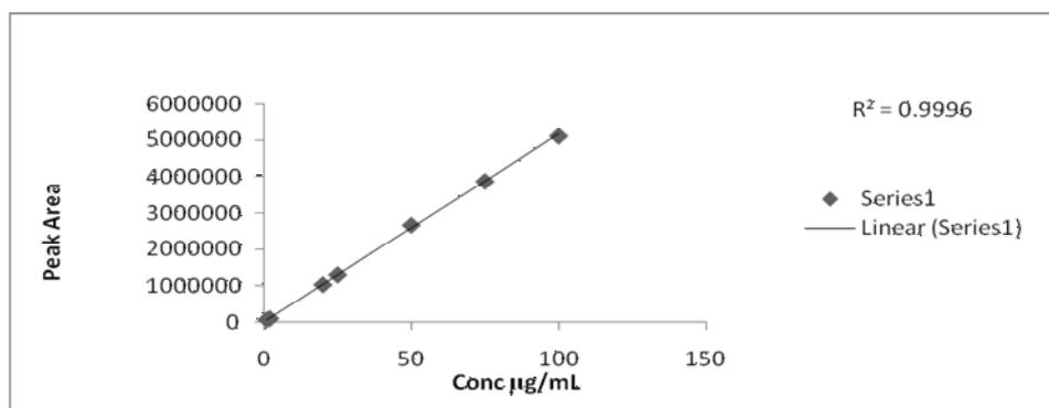
**Figure 2: Linearity curve of Montelukast Sodium**
