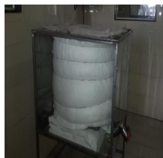
Figure 2: Insulation of Ceramic Fibre Blanket
