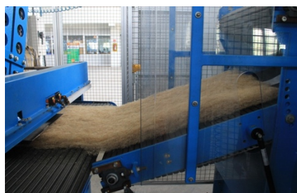
Figure 1. Needle punching of non woven web
