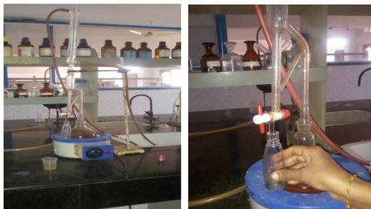
Figure 1: Extraction of cinnamon oil by steam distillation
