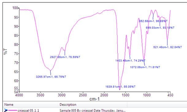
Graph 3: Infrared spectra of compound isolated from FTA 29
