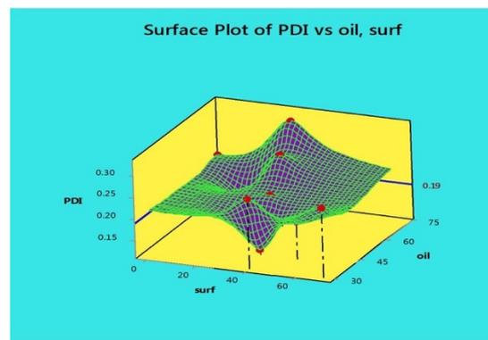
Figure 6: Contour surface plot of PDI vs. surfactant and oil concentration
