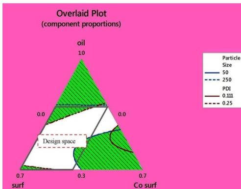
Figure 7: Overlaid plot for particle size and PDI
