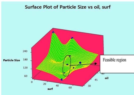
Figure 5: Contour surface plot of particle size vs. surfactant and oil concentration
