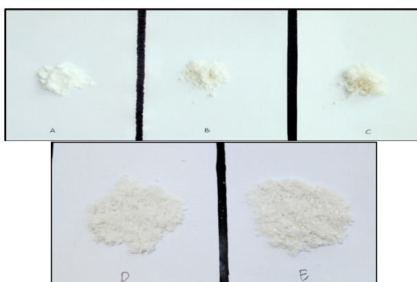
Figure 2: Microcrystalline cellulose (A. Avicel pH 101; B. MCC 1 (Chemically); C. MCC 2 (Enzymatic 5%); D. MCC 3 (Enzymatic 10%); E. MCC 4 (Enzymatic 15%))
