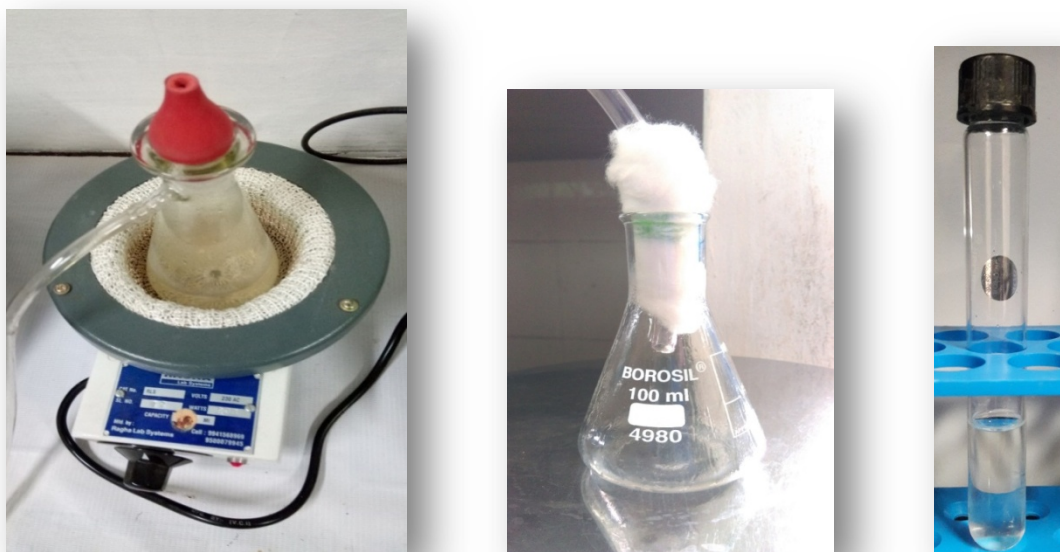
Figure 5: Methanol separation using simple handmade distillation apparatus
