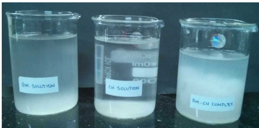
Plate no 1: Polyelectrolyte complex formation between gum karaya and chitosan (GK- gum karaya, CH- chitosan)
