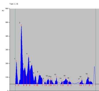
Figure 7: Chromatogram of extract at 366 nm (Track 2)
