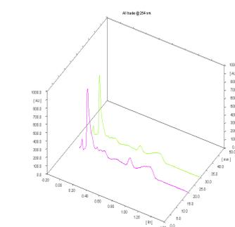
**Figure 3: Chromatogram of extract at 254 nm (Track 1)**
