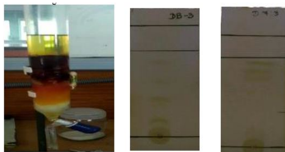
Figure 1: (a) column fractionation of the sample; (b) TLC plate of the crude & (c) TLC plate of fractionate
