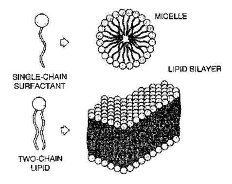
Figure 1: Structure of Micelle and lipid bilayers
